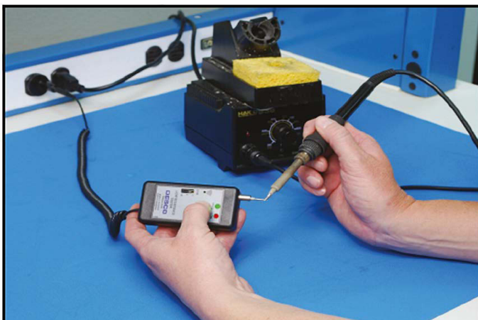
Figure 4. Testing a soldering iron with the 19249 tester
