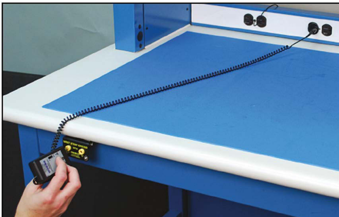
Figure 3. Testing ground points with the 19249 tester
