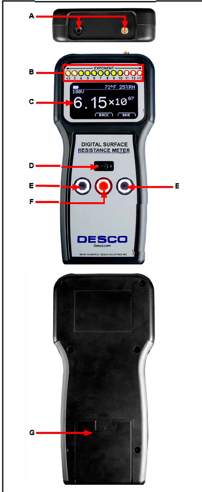
Figure 4. Digital Surface Resistance Meter features and components
