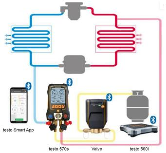
In combination with **testo 560i** and the **testo Smart Valve** the **testo 570s** offers multiple functions to charge refrigerant systems.
