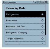
3 Press [▲] / [▼] to select Pressure Leak Test and press [Menu/Enter] to confirm.
