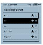
9.2 Setting the refrigerant: Press [▲] or [▼] to select the refrigerant and press [Menu/Enter] to confirm.
