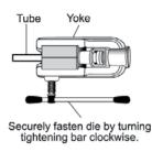
4) Grasp the yoke and rotate the hydraulic cylinder clockwise until it stops. (The adapter should engage the die.)
