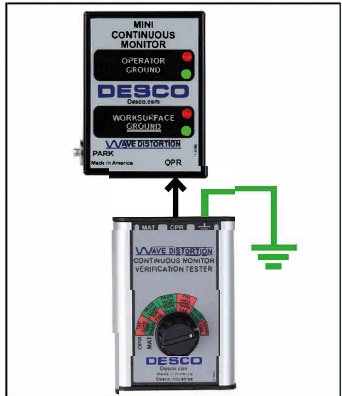
Figure 4. Connecting the Wave Distortion Monitor Verification Tester to the Mini Monitor's operator jack
