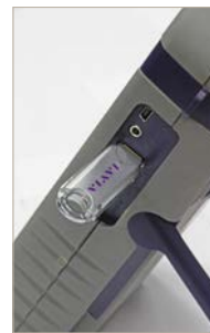
USB flash drive supports transferring test results
