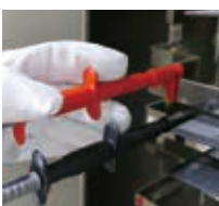
For clamping around the target busbar
