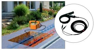
The Easyclamp transmitter clamp is used to send the 33 kHz signal onto and along live cables without shutting off their power. The Easyclamp is connected to the Easyloc TX transmitter and installed around the cable, providing effective route tracing. House connection set for mains power, telephone and cable TV
