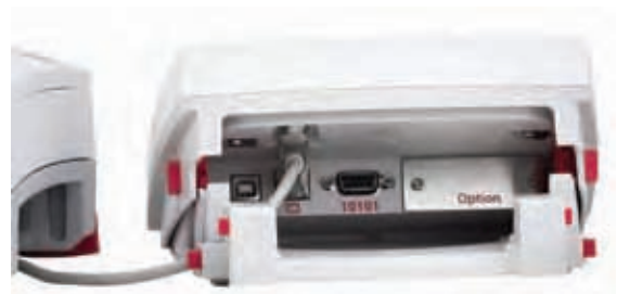
Interface connections on back of Terminal.
