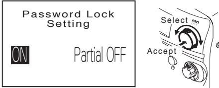
A password is not included when it is shipped from the factory. Immediately after the password lock is activated, it will move to the password input screen.
