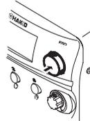
4. When you press the control knob after changing the last digit highlighted in the parameter, the screen will return to the original profile setting screen.
