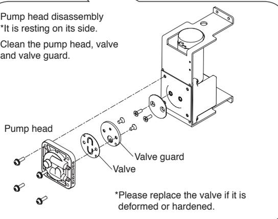
\*Please replace the valve if it is deformed or hardened.
