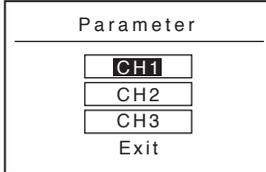
When the channel parameter is selected, the screen shown to the right will be displayed. When you select the channel you want to set here, it will switch to that channel's setting screen.
