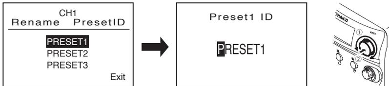
3. Turn the control knob to change the highlighted character in the PRESET NAME, and press the control knob to accept the value and move to the next character.
