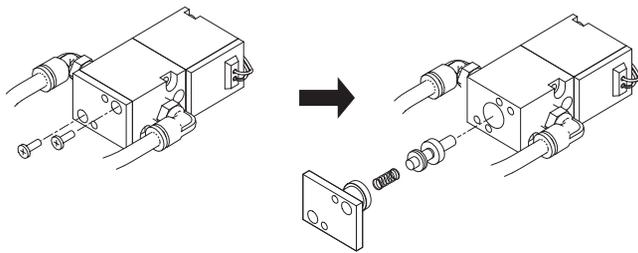
3. Clean the parts that have flux attached to them, such as the inside of the electromagnetic valve, with alcohol.
