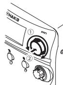
2. When you press the control knob once in the profile setting screen, you can change the value of the profile parameter highlighted.
