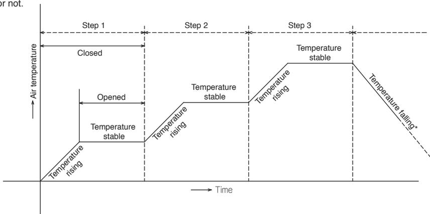
\*In Auto mode, a 15 second cool-down will be performed after all steps are completed and the air will stop.
