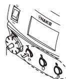
2. Select the item you want to change in the screen above by turning the control knob to highlight the item, and press the control knob to change the setting. When you are finished, turn the control knob to select EXIT and press the control knob.
