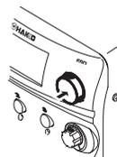
3. To change the parameter value, turn the control knob to highlight the value you want to change, and press the control knob start the change.
