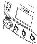
2. By turning the control knob, the preset temperature to be selected will change.
