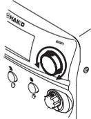
3. Press the control knob when the desired preset temperature is highlighted.
