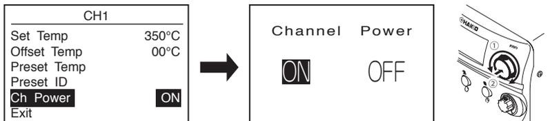
2. When you select either ON or OFF for the CHANNEL POWER and press the control knob, it will return to the setting screen. At this time, if you set the power to OFF, the setting screen will be as shown below. This is because settings other than the channel power are no longer necessary.
