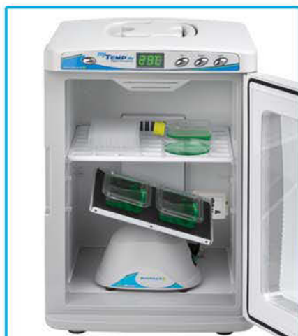
MyTemp Mini shown with H3D1020 (Rocker settings are fixed to 24rpm and 20° tilt)
