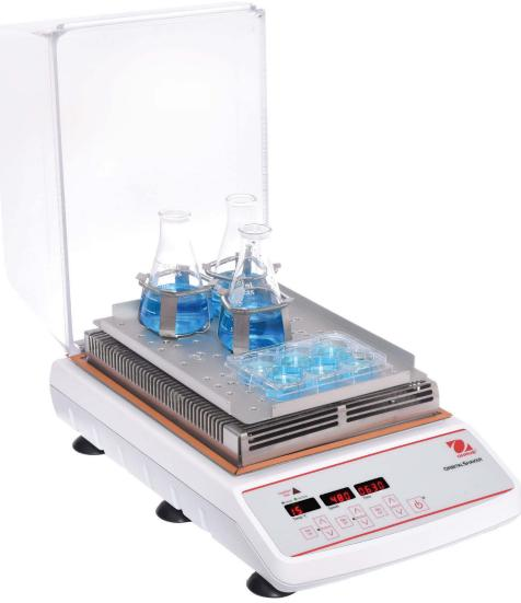
OHAUS Incubating Light Duty Shakers are designed to incubate samples from 10°C below ambient to 65°C depending on the model. The Incubating Mini Shaker has an 8 lb (3.6 kg) capacity while the Incubating Microplate Shaker can hold up to four standard or deep well plates. Incubating-Cooling Mini Shaker is designed to hold two microplates or two optional modular tube blocks. All models feature LED displays with touchpad controls.
