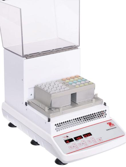
OHAUS Incubating Cooling Orbital Shakers are designed to incubate samples from 10°C below ambient to 65°C. Incubating Cooling Mini Shaker is designed to hold two microplates or two optional modular tube blocks in a variety of configurations. All models feature touchpad controls with easy-to-read, independent LED displays for temperature, speed and time. Microprocessor control provides consistent uniform shaking action.
