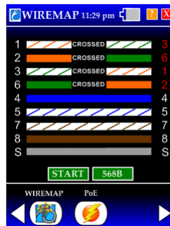
Example - Crossed 12-36 shielded cable
