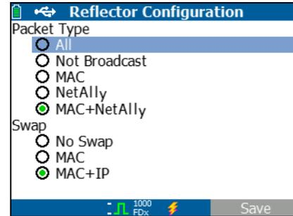
Figure 12. Reflector Default Configuration Screen
