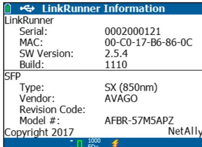
Figure 13. LinkRunner Information Screen with Connected Fiber Adapter
