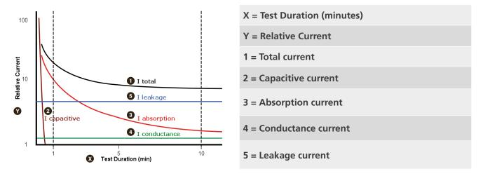
In the case of dry insulation, conductance current may be negligible and the leakage current may be low, in which case the absorption current will dominate the total current measured.
