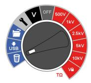
There are two delete functions; delete a single result and delete all results. Select the bin icon on the central rotary switch. The first record indicated contains the result of the last test performed. Up / down arrows navigate through records and the OK button is used to select delete where the 'X' changes to a tick and the on screen bin icon flashes. A subsequent press of the OK button activates the deletion.
