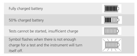
When mains power is present the indicator shows the battery is being charged by animating the segments of the bar graph.
