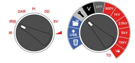
A timed test IR(t) will automatically terminate an insulation test after a preset time. Default timer is set to 1 minute and is adjustable within the settings function. This is a useful feature which saves the user watching the display for the full duration of the test and the possibility of missing the 1 minute reading.
