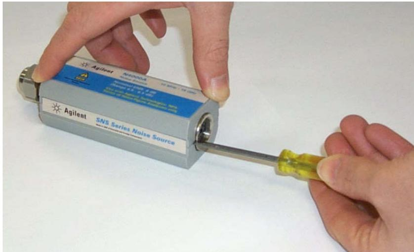
Disassemble the Smart Noise Source by performing the following steps.
