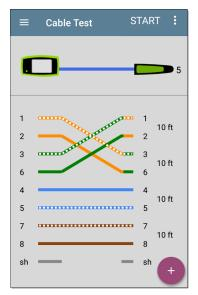
The image above indicates a crossover between pairs 1, 2 and 3, 6 and a WireView accessory number 5. The last row of WireView results indicates whether the cable is shielded: an unbroken line between **sh** means a shielded cable is detected.
