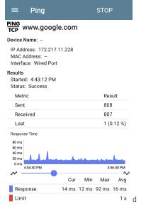
The graphs update in real time and then save and display data for up to 24 hours (depending on test type and/or link status). A legend indicates the measurements that correspond to each plotted color.
