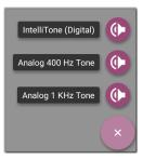
Select a Tone option from the menu. The LRAT 3000-4000 emits the tone through the cable, and the probe detects it, allowing you to trace the wire or locate it in a switch closet or rack.
