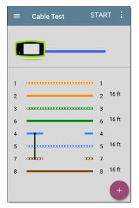
This unterminated cable test image shows a shorted cable between pins 4 and 7.
