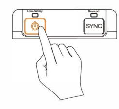
Press for 1 second to turn on the scale. Press for 2 seconds to turn off the scale. 4. Scale keypad On/Off Operation.
