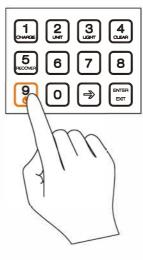
Press of for 2 seconds to turn on the scale keypad.
