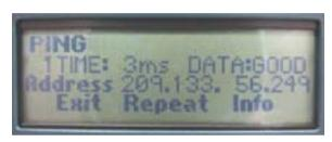
PINGER PLUS+ displays results of a PING to a remote device. The MAC Address is displayed by pressing Info key.
