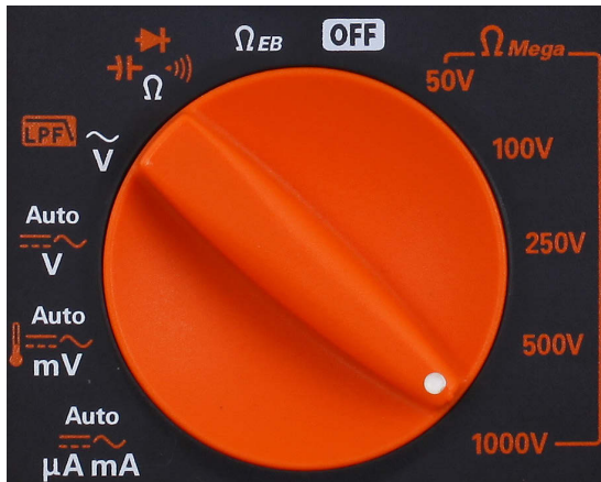
Figure 6. Insulation resistance tester with full featured DMM
