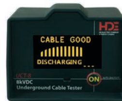
Good cable test results - cable discharging
