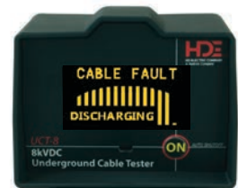
Faulted cable test results - cable discharging
